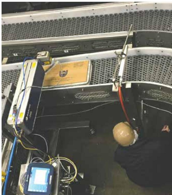
The system is based on marking with a CO2 laser which works without compromising the waxed layer or the paper. The marking of the fish block is created between the wax and paper with a special food safe ink that reacts with the laser, thereby permanently marking the blocks with for instance details about product type, time of production, batch codes, barcodes or QR codes.
